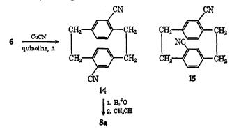
6, by its conversion to the same dicarbomethoxy derivative 8a. Subsequent elegant studies made by Cram and coworkers on this reaction and other related reactions culminated in the finding<sup>20</sup> that the other isomer is 15, formed by a mechanism of "ring opening" in which either 6 or 14 splits open at one of the cyclophane bridges followed by rotation of one of the benzene rings and subsequent closure of the bridge.
