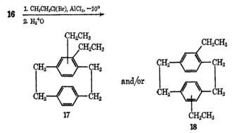
elucidated. However, based on a finding that no detectable amount of the unsubstituted poly(p-xylylene)(3) was isolated upon polymerization of the diethylated [2.2]paracyclophane, it is probable that the diethylated product consists mainly of 18 and not the expected 17 (see Scheme II); this is possible only through close transannular interaction between the two benzene rings.
